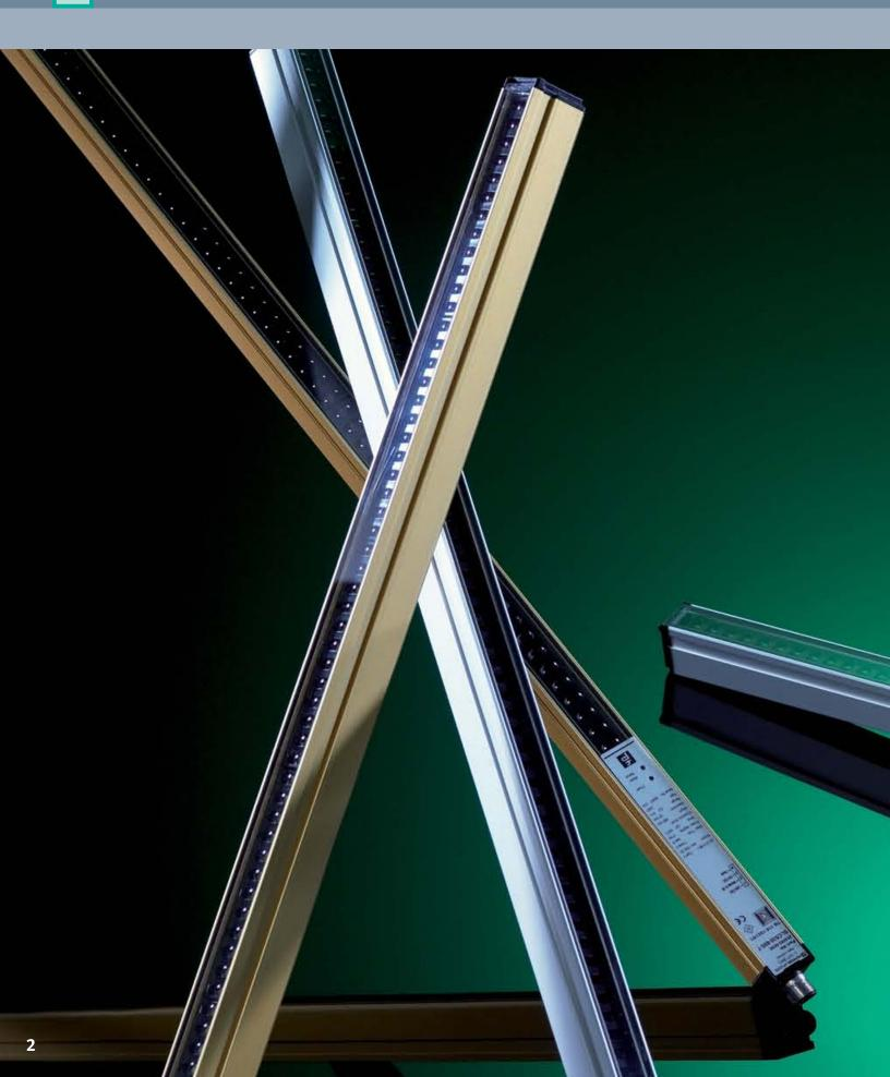
High resolution, ultra-slim safety light curtains are the ideal solution for the most challenging machine safety applications. Higher resolution (smaller beam spacing) reduces the safety mounting distance with respect to the point-of-operation hazard, while the extremely small footprint (only 20 mm wide by 30 mm deep!) offers unsurpassed mounting flexibility.
